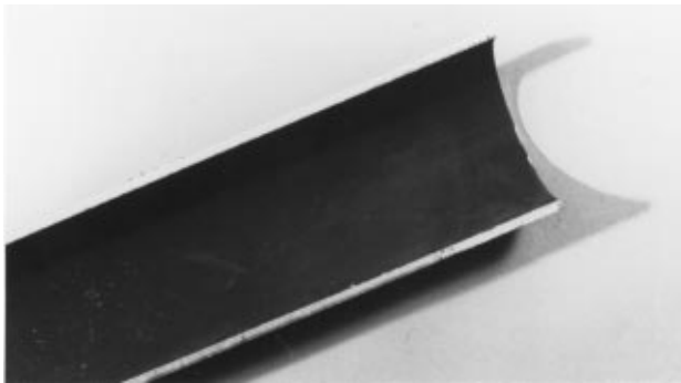
Figure 7 — Passivated pipe surface
