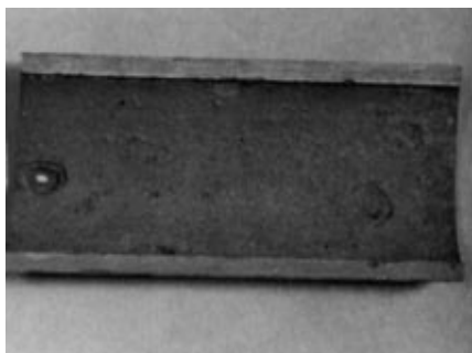
Figure 1 — Oxygen attack occurs as a distinctive pit formation
